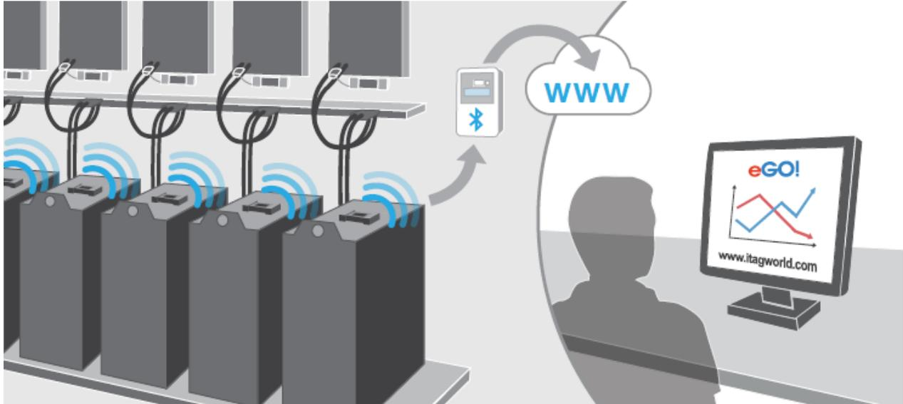
**The eGO! battery monitor measures individual battery performance, helping prevent costly battery damage.**
